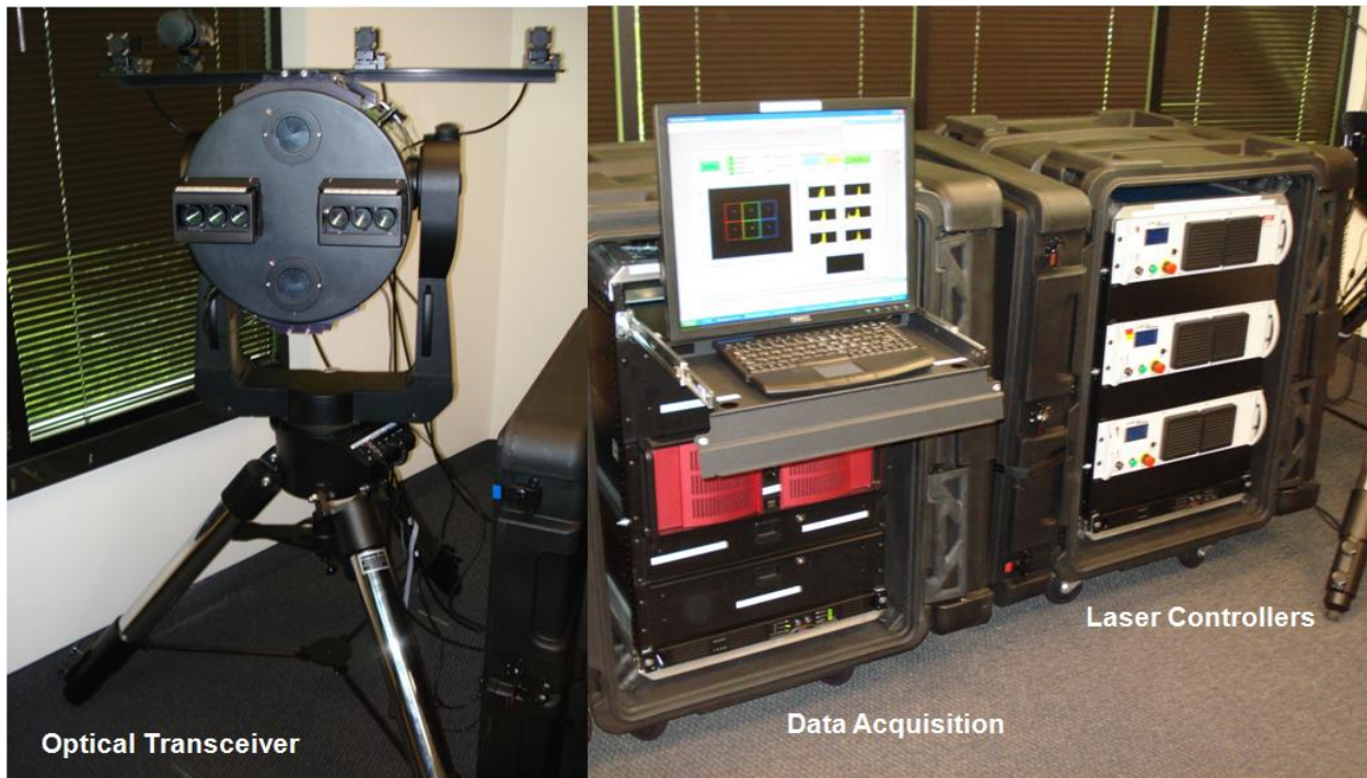
Figure 1. Optical, laser, and computer hardware comprising each REAP terminal.
